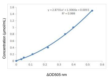
Figure 1. Standard curve for GOT
